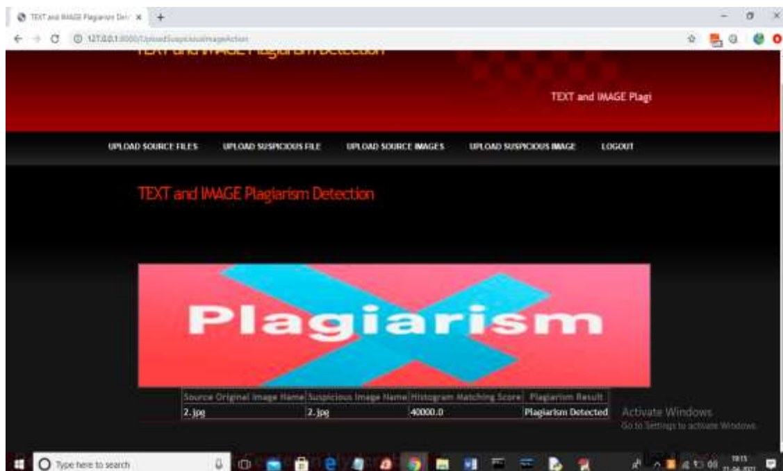
Fig 6: In above screen histogram matching score is 40000 which means all pixels matched so plagiarism is detected in above result.
